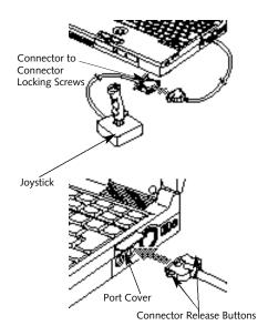
Figure 4-13 Installing a MIDI/joystick Device
